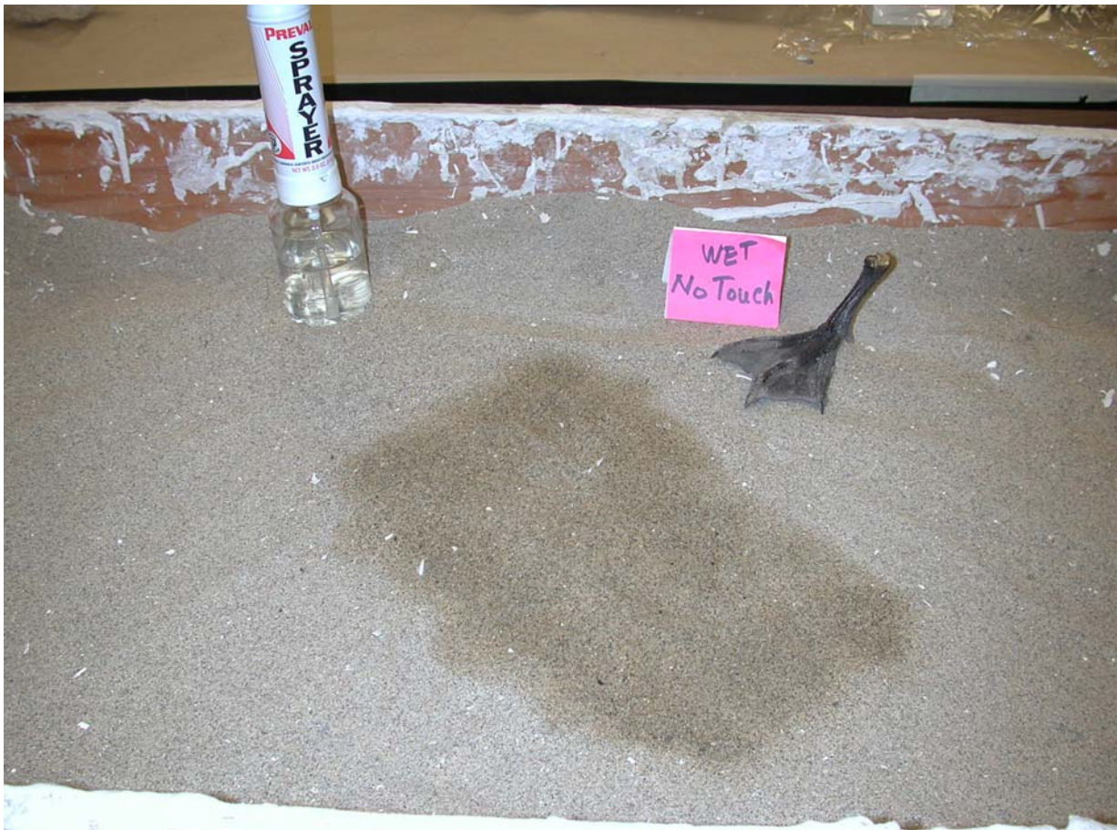
Fig. 1 - Two footprints using a duck foot have been made in the sand. Steps 1 and 2 have been completed. The darker color of the sediment indicates that the material is not dry yet and cannot be lifted from the adjacent sediment.
