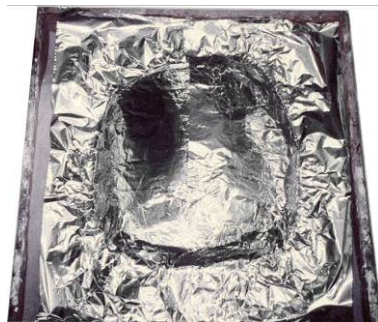
Figure 6: The specimen and flange covered in foil and ready for the clay layer.
