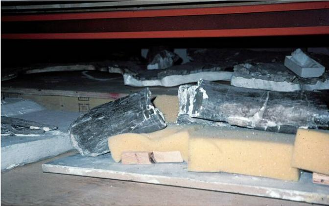
Figure 1: Failure of an ancient plaster bond on a sauropod tibia lying on inadequate support in the collections.
