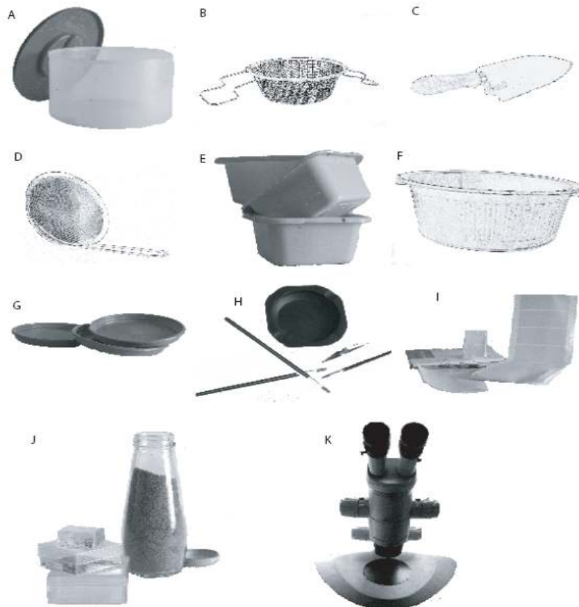
Figure 1. Materials used for sieving: A-- transparent bowls used to dissolve the boulders collected in the field; B- 15000µm sieve; C-garden shovel used to move sediment between bowls; D- 750µm sieve; E- various small-sized bowls (30x30cm); F- large-sized bowl (30cm diameter); G-trays to dry sediment; H- painted ashtray for picking, and various brushes; I- labeling material; J- small transparent boxes used to store sorted specimens and glass juice bottle used to store unpicked sediment; K- binocular microscope.
