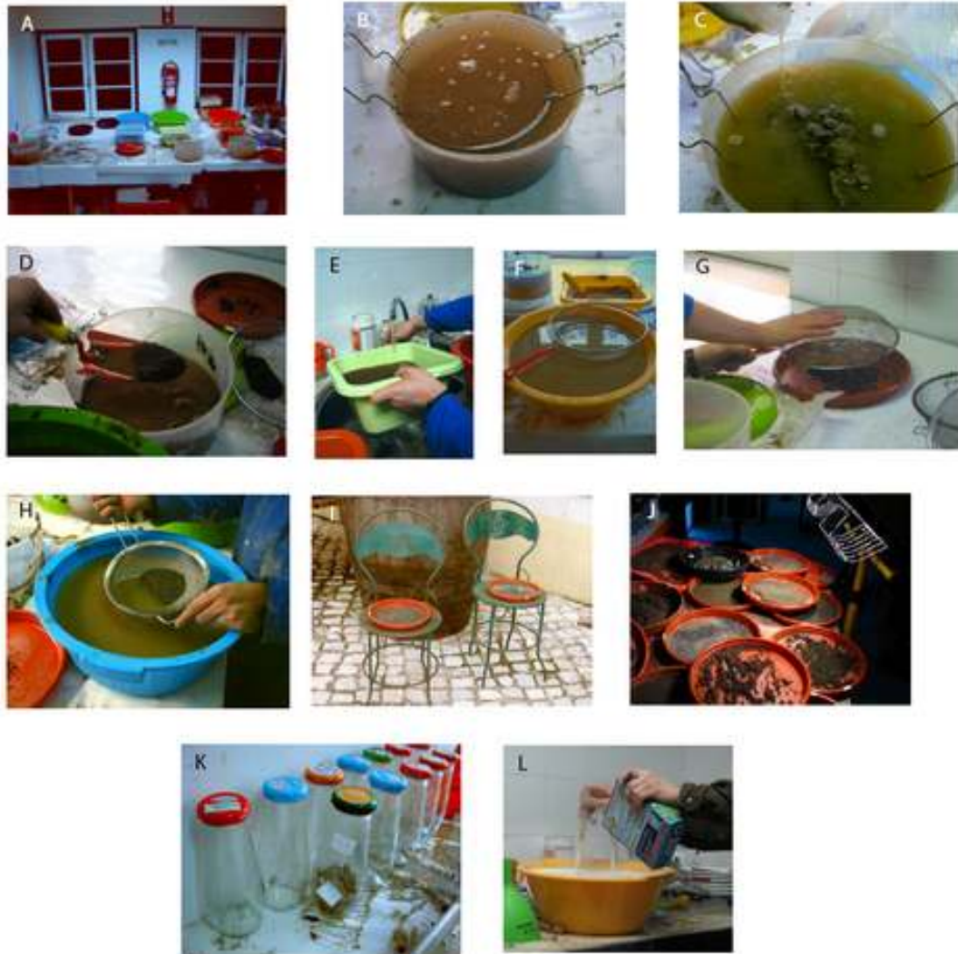
Figure 2. Some aspects of the sieving methodology: A-- Lab during the sieving season (note the different colored bowls), B-- the clay boulders are left to disaggregation in the 1500µm sieves, C-- a dose of hydrogen peroxide can be added if the boulders are hard to dissolve, D-- with a garden shovel the sediment is transferred to the 750µm sieve, E-- the bowl to which the sieved sediment will go to can be filled with cold water, F-- sediment passes through the sieve with circular movements in the water, G-- in order to minimize the amount of time sieving, small parcels of sediment should be done at a time, H-- sediment passes through the 500µm sieve, I-- the sediment is left to dry at atmospheric conditions, J-- if the weather does not permit the sieved sediment can be left to dry under strong light, K-- store the dried sediment in juice glass bottles, L-- by the end of the day clean the pipes using deflocculating agents and hot water.
